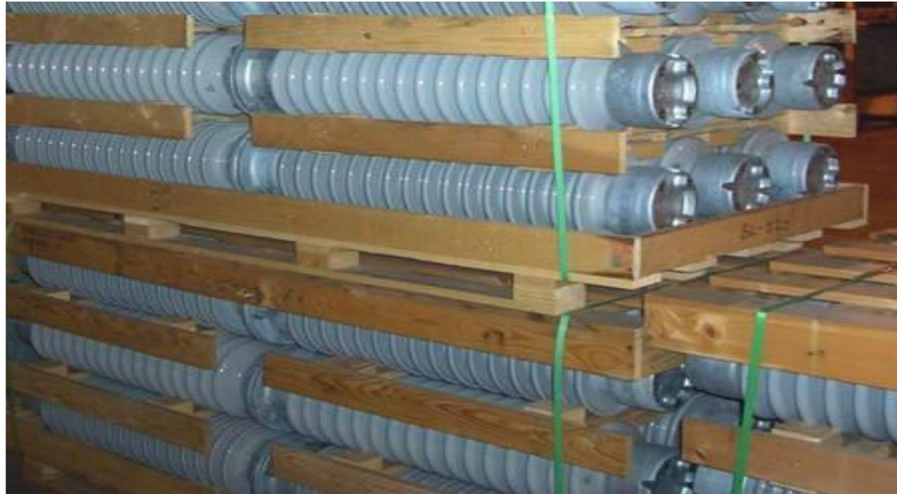
**Aesthetic, all-weather packing after due cleaning of Insulators**
