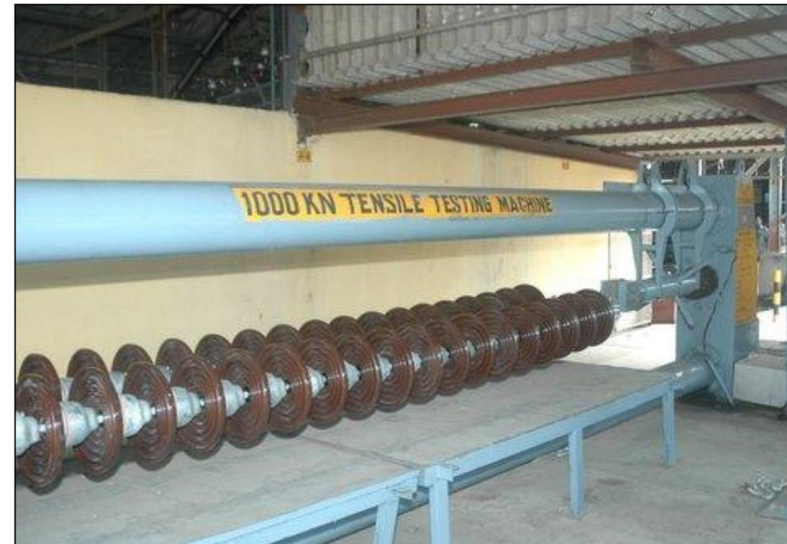
1000kN Tensile Testing Machine
