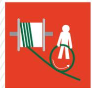
Removal of a twist by this method is performed by one person. To do this, create a spiral from the cable wound on the drum and roll / unscrew it to the free end of the cable. Depending on the turn, rolling / unscrewing should be done to the right or left. Repeat these steps if the turn has not been eliminated after the first attempt.
