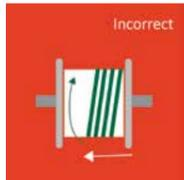
Crane cables of the TFCrane series may be produced in a left, or right-hand direction, therefore we recommend to contact with TFK engineers to determine the direct way of winding. This will allow you to take advantage of the natural tendency of the cable to move to the left/right when it is rewound and keep the scrolls close to each other.
