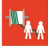
This method requires the involvement of two people who, holding the roller on which the cable is placed, move towards the free end of the cable, thereby shifting the „wave“ of the turn. This operation should be performed until the effect of turning is completely removed.
