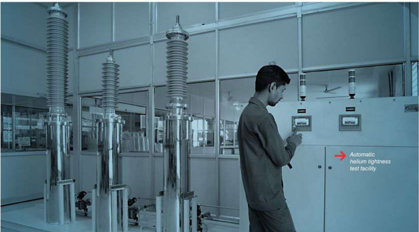
Shielded HV test lab capable of all routine tests as per IEC '137
