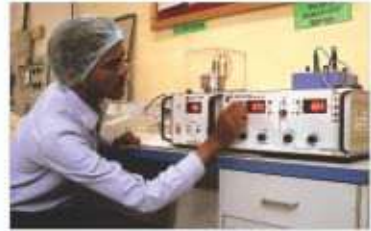
State-of-the-art oil test lab capable of testing oil PPM, BDV, Tan & IR
