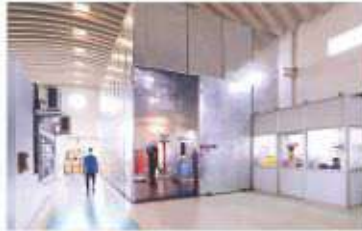
Shielded HV test lab capable of all routine tests as per IEC '137
